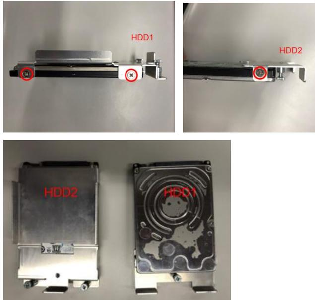
**Step 7** Insert and screw the HDD1 module into the HDD bay.
