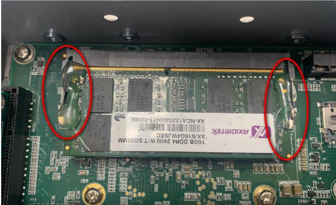
**Step 7** Stick thermal pad onto DDR (option)
