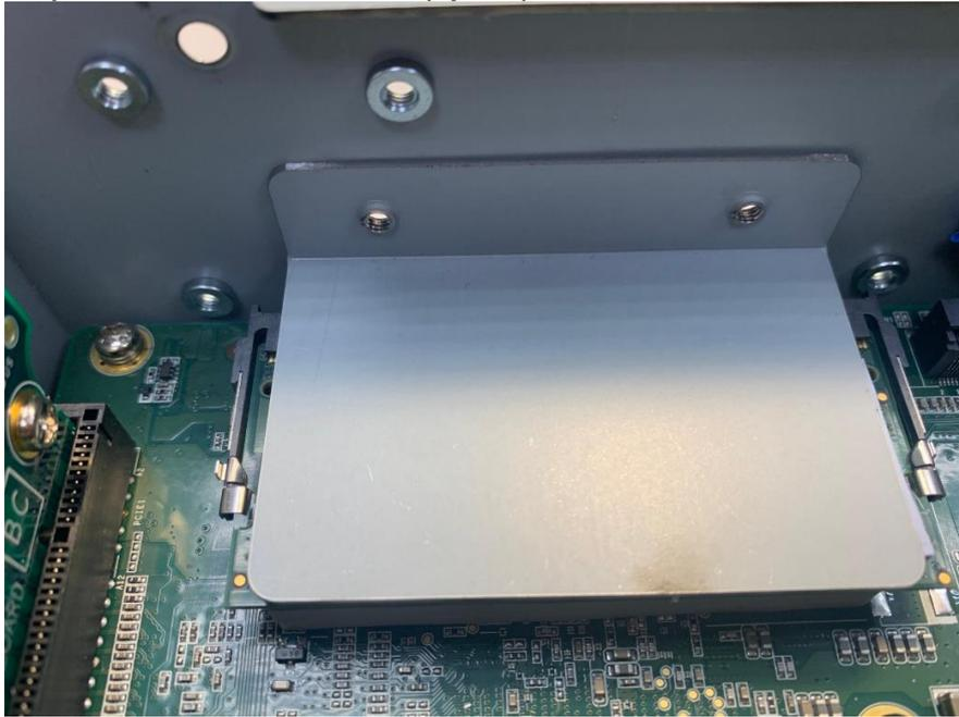
**Step 9 Put the screw of Bracket (option)**
