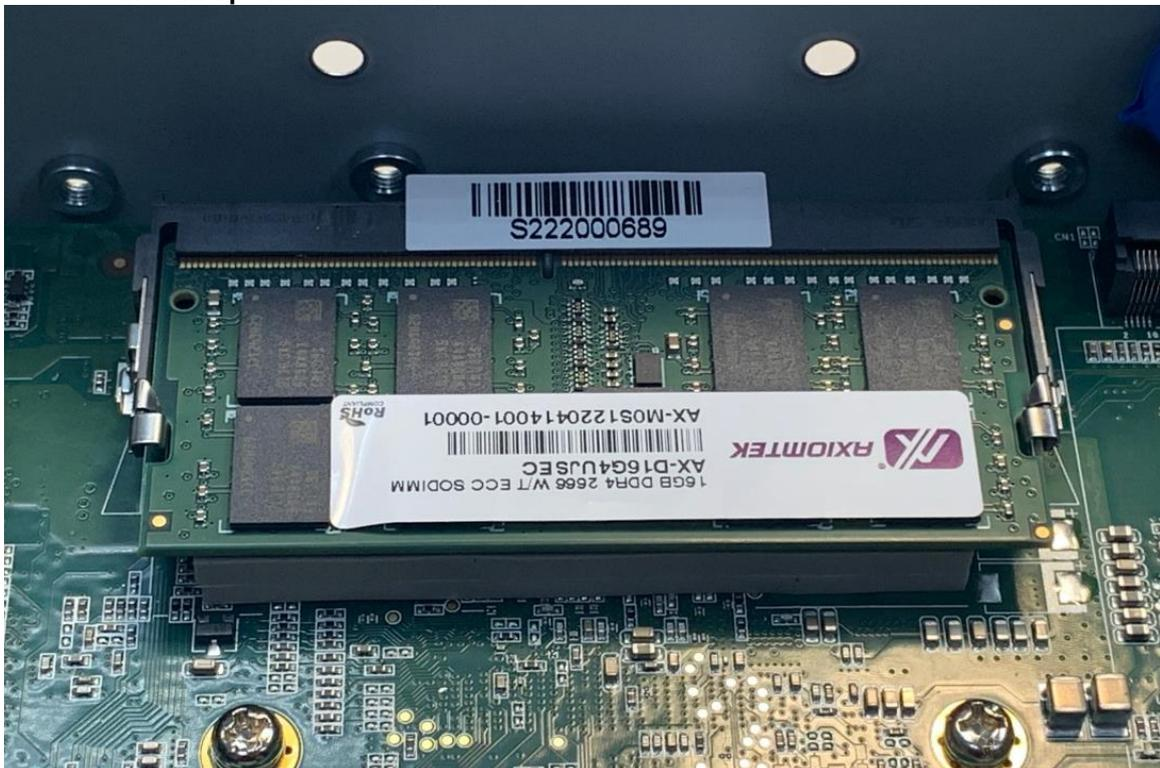
**Step 6** The memory module is locked by two latches on the sides. But we still strongly recommend using “LDC737” silicone on the two sides of the memory for anti-vibration.
