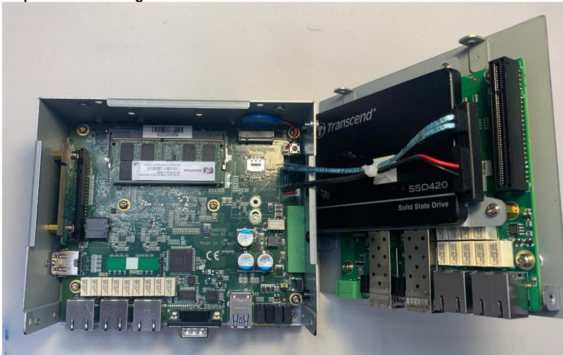
**Step 7** Put the cover back to the system, and tighten screws to close the chassis.
