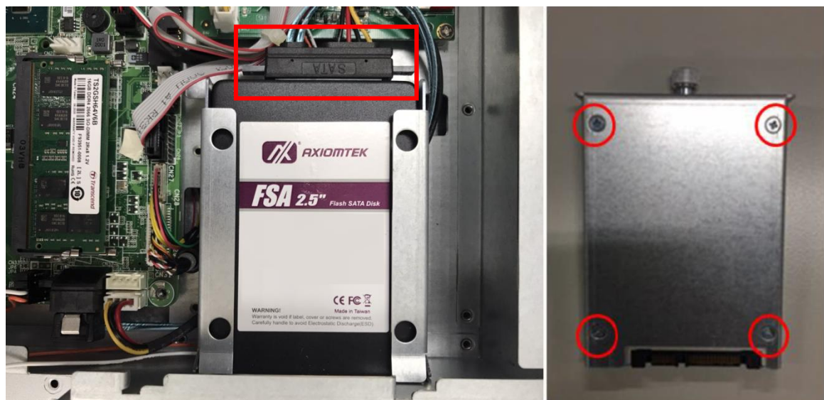
Figure 2-14: Fasten an HDD to the bracket and plug in the "SATA + Power" connector
