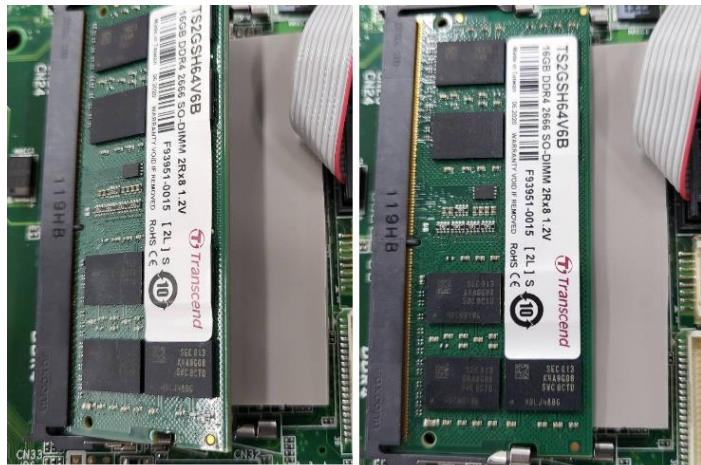
Figure 2-18: Installing a memory module
