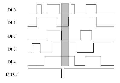
The source signals meet the defined conditions and trigger the AX92351 to send an INT0 interrupt signal.
